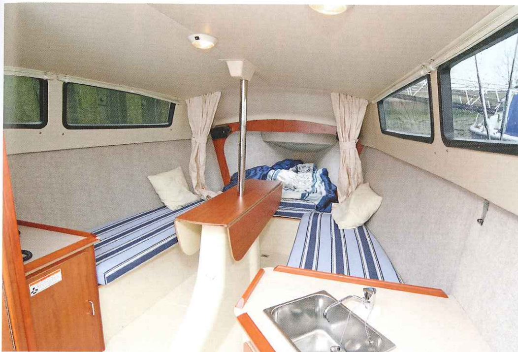
An open-plan interior, formed by a full internal moulding and with the water-ballast tank beneath the sole
