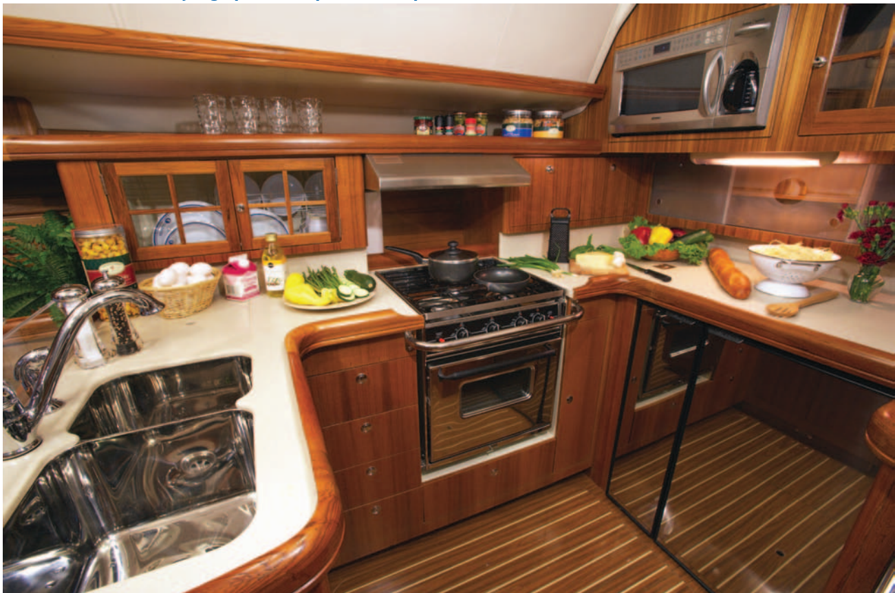
Galley high points: Ample counter space and a fiddle that doubles as a handhold
