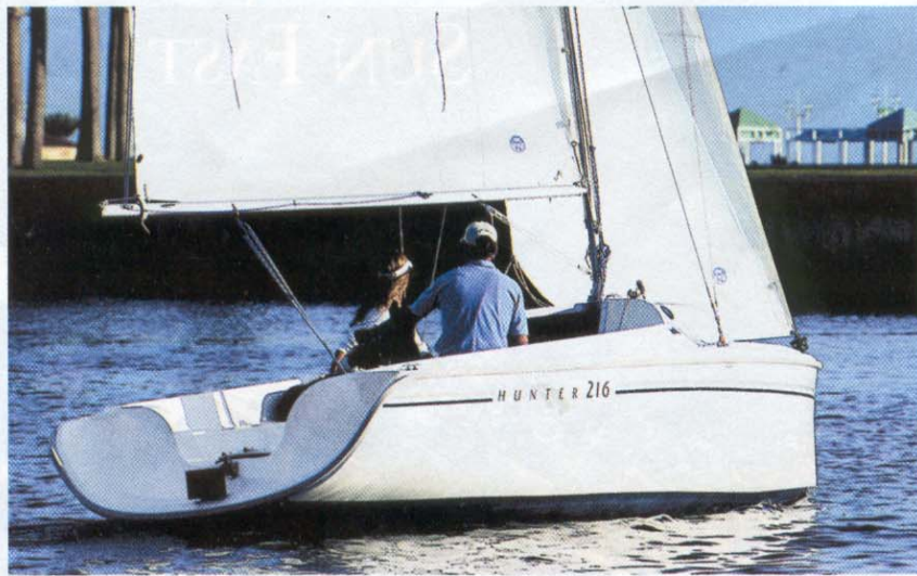
HUNTER'S 21-FOOT PERFORMANCE daysailer has room in its cockpit to take a family of four around the bay and around the buoys. A hydraulic pump hidden below the cockpit floor (right) raises the 500-pound centerboard.
