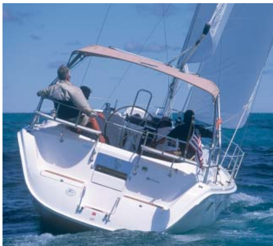
The B&R rig eliminates the backstay and a stainless steel arch raises the traveler off the cockpit sole, opening up the cockpit.
