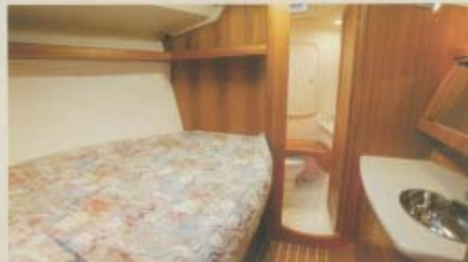
The forecabin has standing room for two people, with a washbasin and adjacent heads/shower compartment. Ventilation is through the hatch only
