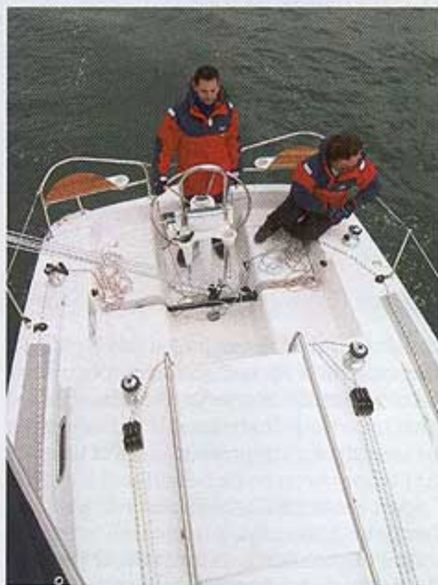
▲ The Legend 27 is one of the smallest boats in the UK to have wheel steering as standard
