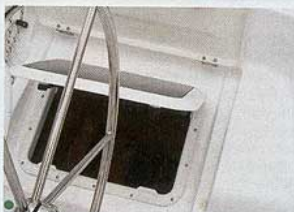
▲ Lifting the starboard cockpit seat beside the wheel reveals the aft cabin hatch
