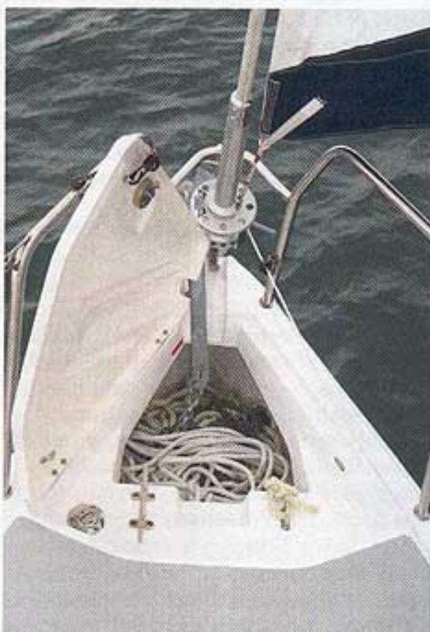
▲ Reasonable anchoring provision, but detailed changes will be seen on production boats
