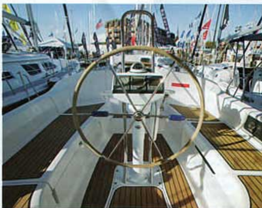
Lewmar's 36-inch folding wheel is a neat solution to the problem of opening access from the swim platform through the cockpit and into the companionway.
