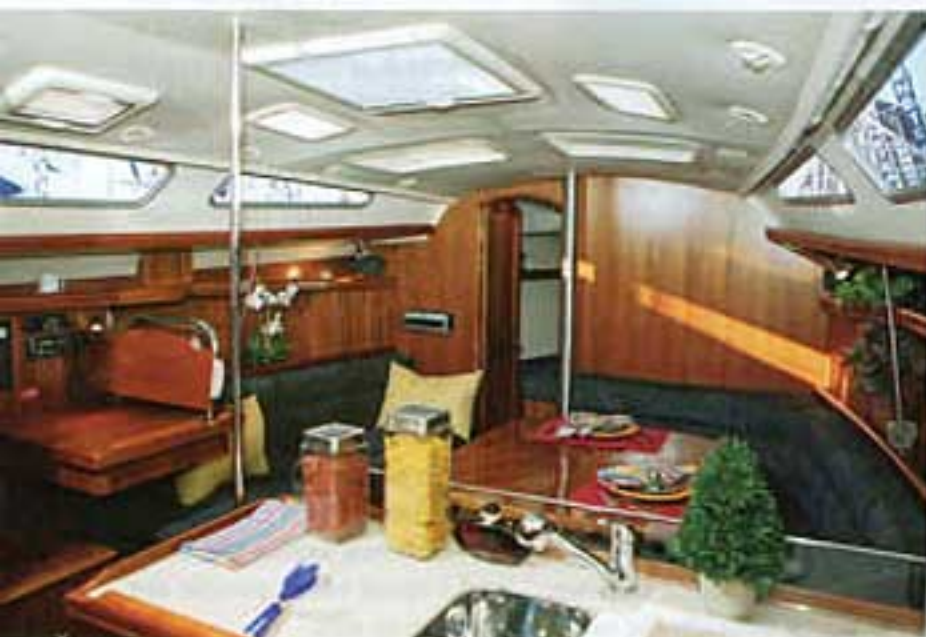
With stainless-steel tie-rods and posts supporting the rig and deck—and with plenty of portlights and hatches in the overhead—the Hunter's interior is especially light and open.
